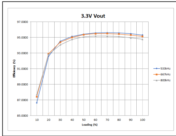
Figure 11: LGA110D-01DADJJB Efficiency Curves at different switching frequency @ 25°C, Vin = 12V Loading: I o = 10% increment to 80A
