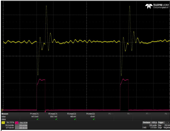
Figure 44: LGA110D-01DADJJ Transient Response – Vo Deviation 25% to 75% to 25% load, 100 A/uS slew rate, V_{IN} = 12 Vdc V_O = 0.5 V Ch 1: I_O Ch 2: V_O f_{SW} = 500 KHz
