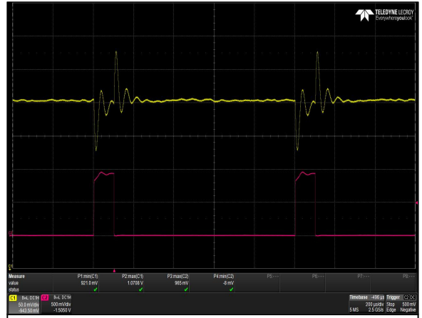
Figure 45: LGA110D-01DADJJ Transient Response – Vo Deviation 25% to 75% to 25% load, 100 A/uS slew rate, V_{IN} = 12 Vdc V_O = 1 V Ch 1: I_O Ch 2: V_O f_{SW} = 500 KHz
