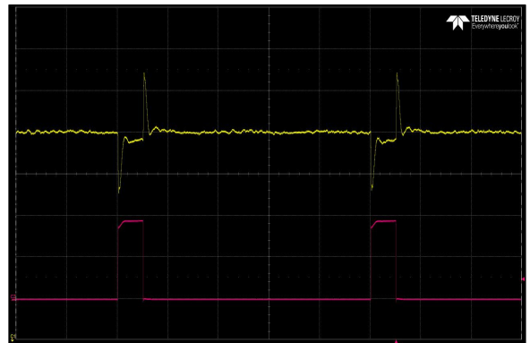
Figure 43: LGA110D-01DADJJ Transient Response – Vo Deviation 25% to 75% to 25% load, 100 A/uS slew rate, V IN = 12 Vdc V O = 1 V Ch 1: I O Ch 2: V O f SW = 500 KHz
