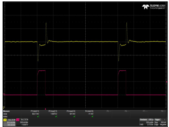
Figure 47: LGA110D-01DADJJ Transient Response – Vo Deviation 25% to 75% to 25% load, 100 A/uS slew rate, V_{IN} = 12 Vdc V_O = 1 V Ch 1: I_O Ch 2: V_O f_{SW} = 500 KHz
