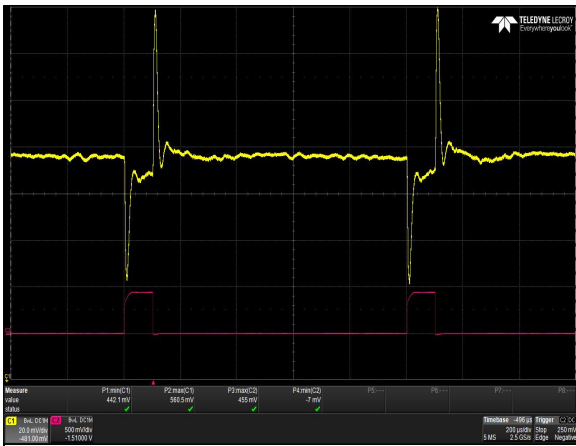
Figure 46: LGA110D-01DADJJ Transient Response – Vo Deviation 25% to 75% to 25% load, 100 A/uS slew rate, V_{IN} = 12 Vdc V_O = 0.5 V Ch 1: I_O Ch 2: V_O f_{SW} = 500 KHz
