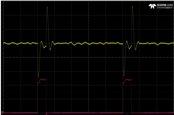
Figure 40: LGA110D-01DADJJ Transient Response – Vo Deviation 25% to 75% to 25% load, 100 A/uS slew rate, V IN = 12 Vdc V O = 0.5 V Ch 1: I O Ch 2: V O f SW = 500 KHz
