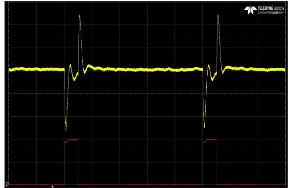
Figure 41: LGA110D-01DADJJ Transient Response – Vo Deviation 25% to 75% to 25% load, 100 A/uS slew rate, V IN = 12 Vdc V O = 1 V Ch 1: I O Ch 2: V O f SW = 500 KHz
