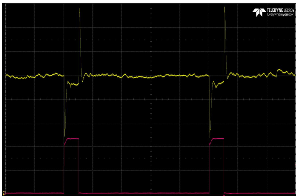
Figure 42: LGA110D-01DADJJ Transient Response – Vo Deviation 25% to 75% to 25% load, 100 A/uS slew rate, V IN = 12 Vdc V O = 0.5 V Ch 1: I O Ch 2: V O f SW = 500 KHz
