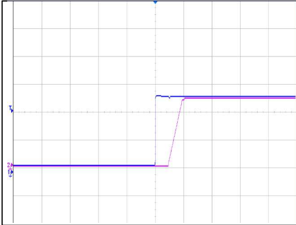
Figure 7: BDQ1300-48S12B-4L Output voltage startup by power on (50mS/div) V_{IN}=54V, I_O=107A Ch 1: V_{IN} (20V/div) Ch 2: V_O (5V/div)
