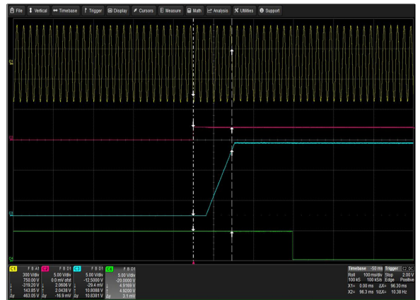
Figure 4: LCM3000L-T Turn-on delay via INH_EN Vin = 264Vac Load: Io = 250A (12V), Isb = 2A Ch 1: Vin Ch 2: INH_EN Ch 3: Vo Ch 4: G_DCOK_C
