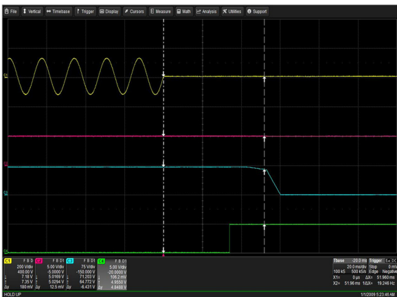
Figure 75: LCM30007-T Hold-up Time Vin = 90Vac Load: lo = 20.8A (72V), Isb = 2A Ch 1: Vin Ch 2: Vsb Ch 3: Vo Ch 4: G_DCOK_C
