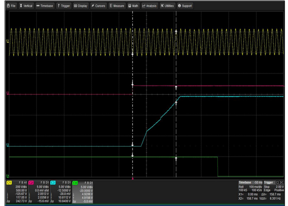
Figure 2: LCM3000L-T Turn-on delay via INH_EN Vin = 90Vac Load: Io = 125A (12V), Isb = 2A Ch 1: Vin Ch 2: INH_EN Ch 3: Vo Ch 4: G_DCOK_C
