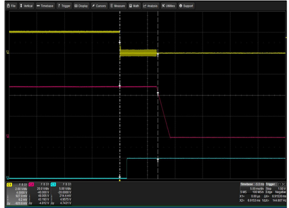
Figure 64: LCM3000W-T Turn Off Characteristic via INH_EN Vin = 264Vac Load: Io = 62.5A (48V), Isb = 2A Ch 1: INH_EN Ch 2: Vo Ch 3: G_DCOK_C
