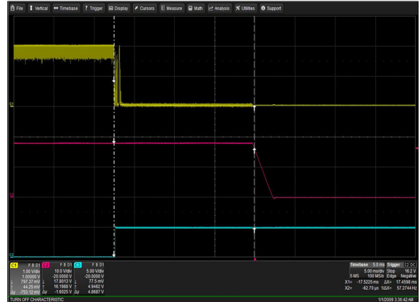
Figure 22: LCM30008-T Turn Off Characteristic via INH_EN Vin = 264Vac Load: Io = 166.7A (18V), Isb = 2A Ch 1: INH_EN Ch 2: Vo Ch 3: G_DCOK_C
