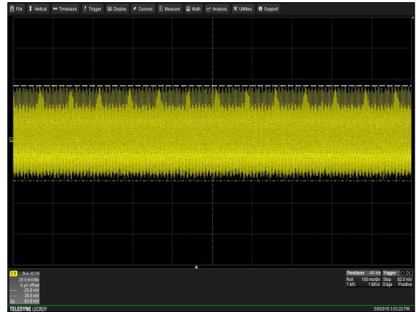
Figure 42: iMP8-3W0-00-A Ripple and Noise Measurement Vin = 230Vac Load: Io = 15.625A Ch 1: V O
