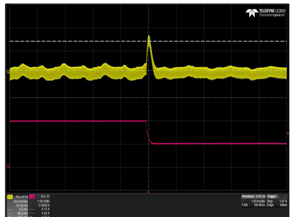
Figure 34: iMP4-1W0-00-A Transient Response - V O Deviation Vin = 230Vac 50% to 25% load change, 1A/μS slew rate Ch 1: V O Ch 2: I O
