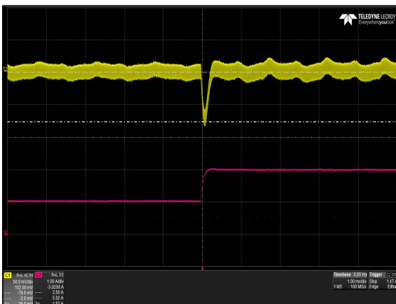
Figure 33: iMP4-1W0-00-A Transient Response - V O Deviation Vin = 230Vac 25% to 50% load change, 1A/μS slew rate Ch 1: V O Ch 2: I O
