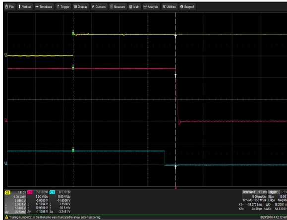
Figure 9: DS2000SPE-3 Turn Off Characteristic via PS_ON_L Load: I O = 78.52A I SB = 3.5A Ch 1: PS_ON_L Ch 2: V O Ch 3: PWOK
