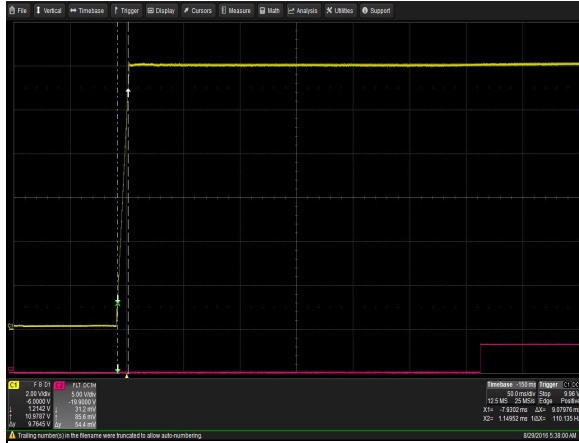
Figure 7: DS2000SPE-3 Output Voltage Startup Characteristic Vin = 90Vac Load: I O = 78.52A I SB = 3.5A Ch 1: V O Ch 2: PWOK
