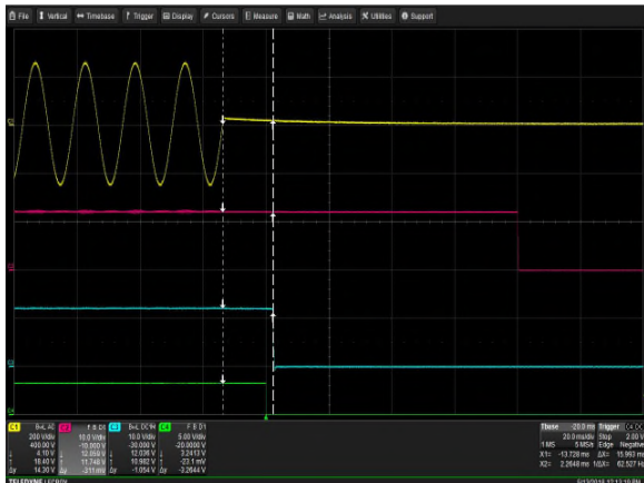
Figure 3: CSV2000BP-3 Hold-up Time - Vin = 180Vac / 63Hz / 0° Full Load: I_o = 163.9A , I_{SB} = 3A Ch 1: AC Mains Ch 2: V SB Ch 3: Vo Ch 4: DC_GOOD / PWOK
