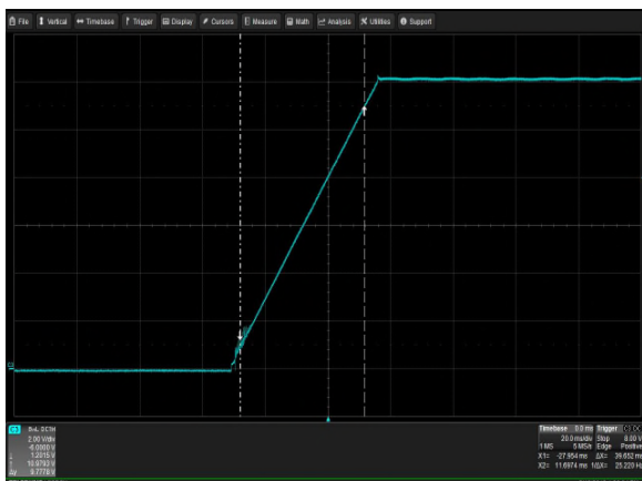
Figure 5: CSV2000BP-3 Output Voltage Startup Characteristic - Vin = 180Vac Full Load: I_o = 163.9A , I_{SB} = 3A Ch 3: Vo
