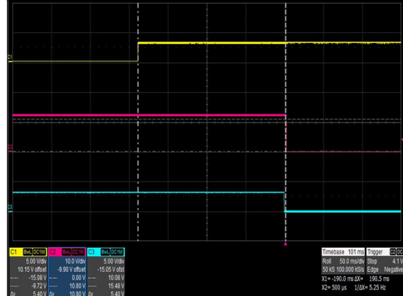
Figure 8: CSV1300BP-3 Turn Off Characteristic via PSKILL Full Load: I_o = 106.6A , I_{SB} = 2.5A Ch 1: PSKILL Ch 2: Vo Ch 3: PWOK
