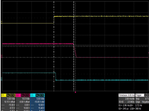
Figure 7: CSV1300BP-3 Turn Off Characteristic via PSRON Full Load: I_o = 106.6A , I_{SB} = 2.5A Ch 1: PSRON Ch 2: Vo Ch 3: PWOK
