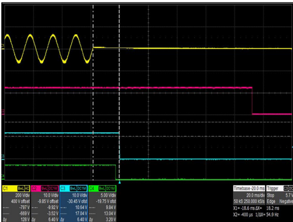
Figure 3: CSV1300BP-3 Hold-up Time - Vin = 90Vac / 63Hz / 0° Full Load: I_o = 73.8A , I_{SB} = 2.5A Ch 1: AC Mains Ch 2: V_{SB} Ch 3: V_o Ch 4: PWOK
