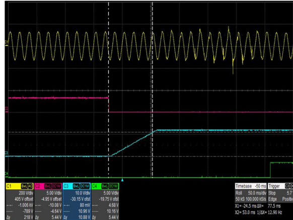
Figure 2: CSV1300BP-3 Turn-on delay via PS_ON - Vin = 90Vac Full Load: I_o = 73.8A , I_{SB} = 2.5A Ch 1: AC Mains Ch 2: PS_ON Ch 3: V_o Ch 4: PWOK
