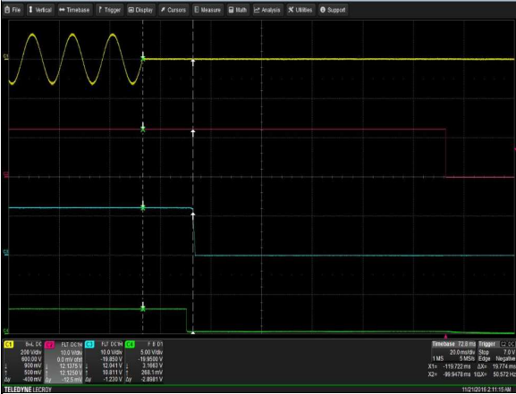
Figure 3: CSU550AP-3 Hold-up Time Vin = 90Vac/63Hz/0° Load: Io = 45A I SB = 2.5A Ch 1: AC Mains Ch 2: V SB Ch 3: V O Ch 4: PWOK
