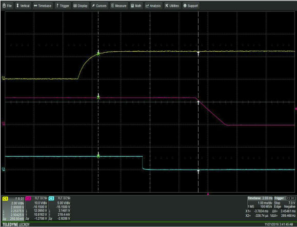
Figure 7: CSU550AP-3 Turn Off Characteristic via PSON Load: I_o = 45A I_{SB} = 2.5A Ch 1: PSON Ch 2: V_o Ch 3: PWOK
