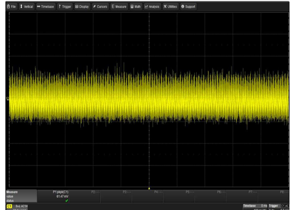
Figure 12: CSU2400AP-3-111 Ripple and Noise Measurement Vin = 218Vac Load: Io = 196.7A I SB = 3.5A Ch 1: V O
