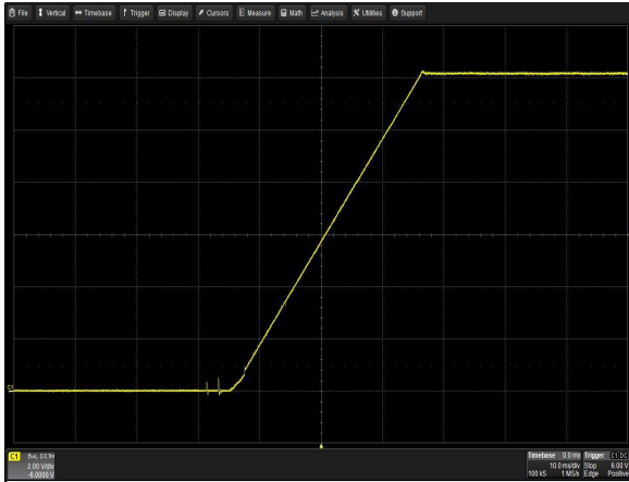
Figure 7: CSU2400AP-3-100 Output Voltage Startup Characteristic Vin = 180Vac Load: Io = 196.7A I SB = 3.5A Ch 1: V o
