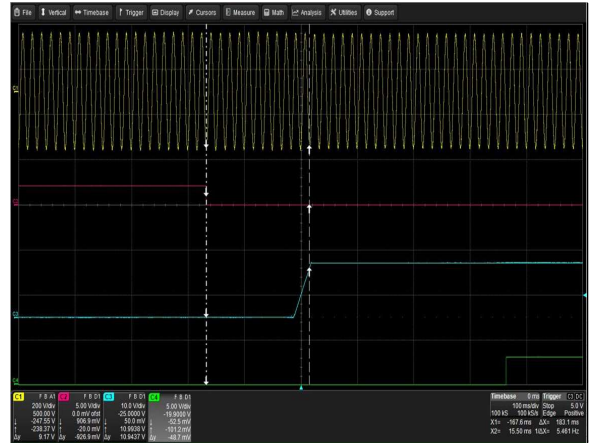
Figure 14: CSU2400AP-3-111 Turn-On Delay via PSON Vin = 180Vac Load: I O = 196.7A I SB = 3.5A Ch 1: AC Mains Ch 2: PSON Ch 3: V O Ch 4: PWOK
