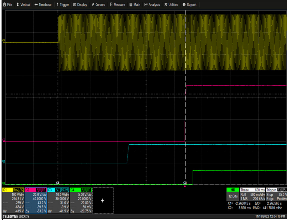
Figure 1: AIF11BAC-01N Turn-On Delay via AC Mains Vin = 90Vac Load: I O = 10.5A I SB = 0.25A Ch 1: AC Mains Ch 2: V O Ch 3: V SB Ch 4: PSU-Good
