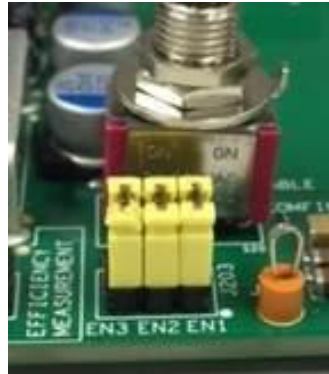
Fig. 9 – The enable jumpers – all 3 shown in place to enable all 3 outputs
