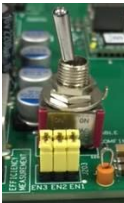
Fig. 4 – Enable jumper location and population
