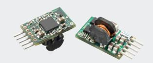
Advanced Energy's Artesyn LDO10C series non-isolated DC-DC converter is designed for cost- and space-sensitive applications. It has a wide 3–13.8 Vdc input range and offers a 0.59–5.1 Vdc adjustable output that accommodates a wide variety of silicon power needs. Capable of delivering up to 10 amps, the converter has a typical efficiency of 94%. A remote enable facility is provided as standard.
