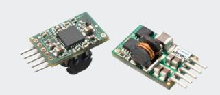
Advanced Energy's Artesyn LDO06C series non-isolated DC-DC converter is designed for cost- and space-sensitive applications. It has a wide 3–13.8 Vdc input range and offers a 0.59–5.1 Vdc adjustable output that accommodates a wide variety of silicon power needs. Capable of delivering up to 6 amps, the converter has a typical efficiency of 92%. A remote enable facility is provided as standard and remote 'power good' indication is available as an option.
