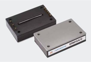
Advanced Energy's Artesyn ERM75W series high performance 75 watt isolated DC-DC converter modules are designed specifically for railway applications. The high input versions feature a 66 to 160 Vdc input that complies with the European EN50155 standard for electronic equipment used on railway rolling stock. There is a choice of four single output models, offering voltages of 5 V, 12 V, 15 V or 24 V.
