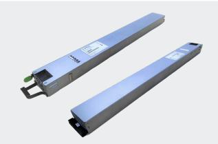
Advanced Energy's Artesyn introduces the 48 V 3 kW ATS PSU for use in the 30 kW EIA 19 Inch Power Shelf (10 + 2) redundant. The PSU is a single-phase AC to DC power supply that operates from nominal input voltage from 187 to 264 VAC and produces 48 V, 62 A (3 kW) DC output, hot-swappable, accurate current sharing and self-cooled. Within the EIA 19 Inch Power Shelf, twelve of the PSUs operate in parallel, current sharing mode to produce 30 kW of 10 + 2 redundant power.
