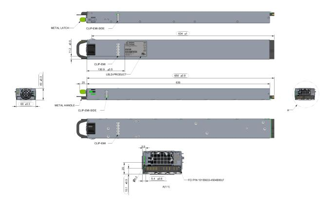
The rear blind-mate connector installed on the PSU is Amphenol FCI 10155633-4504B00LF. This is a R/A plug, PwrBlade ULTRA connector with 4 high power pins, 20 signal pins, and 5 low power pins. Please refer to the drawing below for more details.
