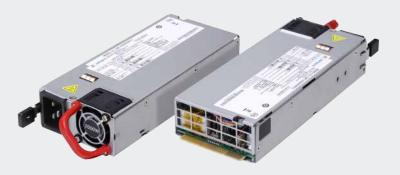
Advanced Energy's Artesyn DS2000SPE is an ultra-high denstiy power supply providing 50W per cubic inch. The 2000 watt DS2000SPE power supply is housed in 1U high rack-mounting enclosures measuring just 3.4 x 7.7 inches (86.3 x 196.5 mm). This form factor is significantly shorter than that of similarly rated earlier-generation power supplies — freeing up valuable system space — and is achieved by use of the latest power switching technology and high density component packaging techniques.
