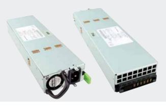
Advanced Energy's Artesyn DS1050 series bulk front end AC-DC power supply accepts a wide range 90–264 Vac input and provides a main 12 V output plus a 3.3 V or 5 V standby output. Rated at 1,050 watts it is an 80 Plus Gold supply with a high half-load efficiency of 92%. Housed in an industry standard 1U x 2U rack-mounting package, the power supply is ideal for space-constrained applications. This series comes in two airflow versions – dc-connector to ac-connector and vice versa.
