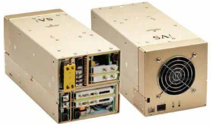
The series offers seven types of modules, including single-, dual- and triple-output units, with individual power outputs of up to 1500 W. The iVS series offers 25 standard output voltages, from 2 Vdc to 60 Vdc, and can provide up to 24 outputs. By connecting modules in parallel and/or series, currents as high as 970 A and voltages as high as 500 V are achievable.
