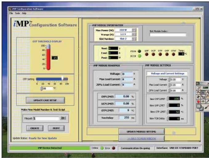
***Digital control of the iMP Series of programmable power supplies from Artesyn Embedded Power extends to configuration of parameters such as over-voltage protection, overcurrent protection and over-temperature protection***
