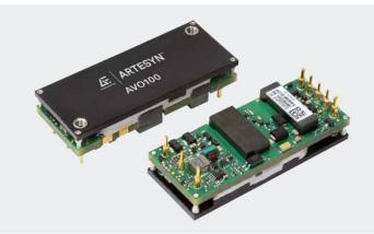
Advanced Energy's Artesyn AVO100-48S28 series isolated DC-DC converter is designed specifically to provide the main 28 Vdc supply for RF power amplifiers in small-cell, low power telecommunications applications.
