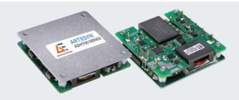
Advanced Energy's Artesyn ADH700-48S50 series half-brick isolated DC-DC converter provides a single regulated low noise output. ADH700-48S50 with 50V/14A output. It has a Telecom input range of 36 to 65VDC and is designed primarily for use with standard 48 VDC telecommunications equipment supplies. The converter's main application area is in low power and remote radio head (RRH) telecommunications applications.
